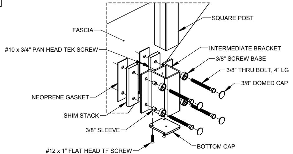
2 TYP. INTERMEDIATE BRACKET MOUNTING CONNECTION
