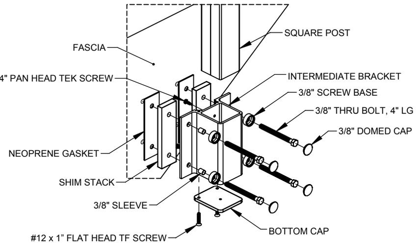
2 TYP. INTERMEDIATE BRACKET MOUNTING CONNECTION
